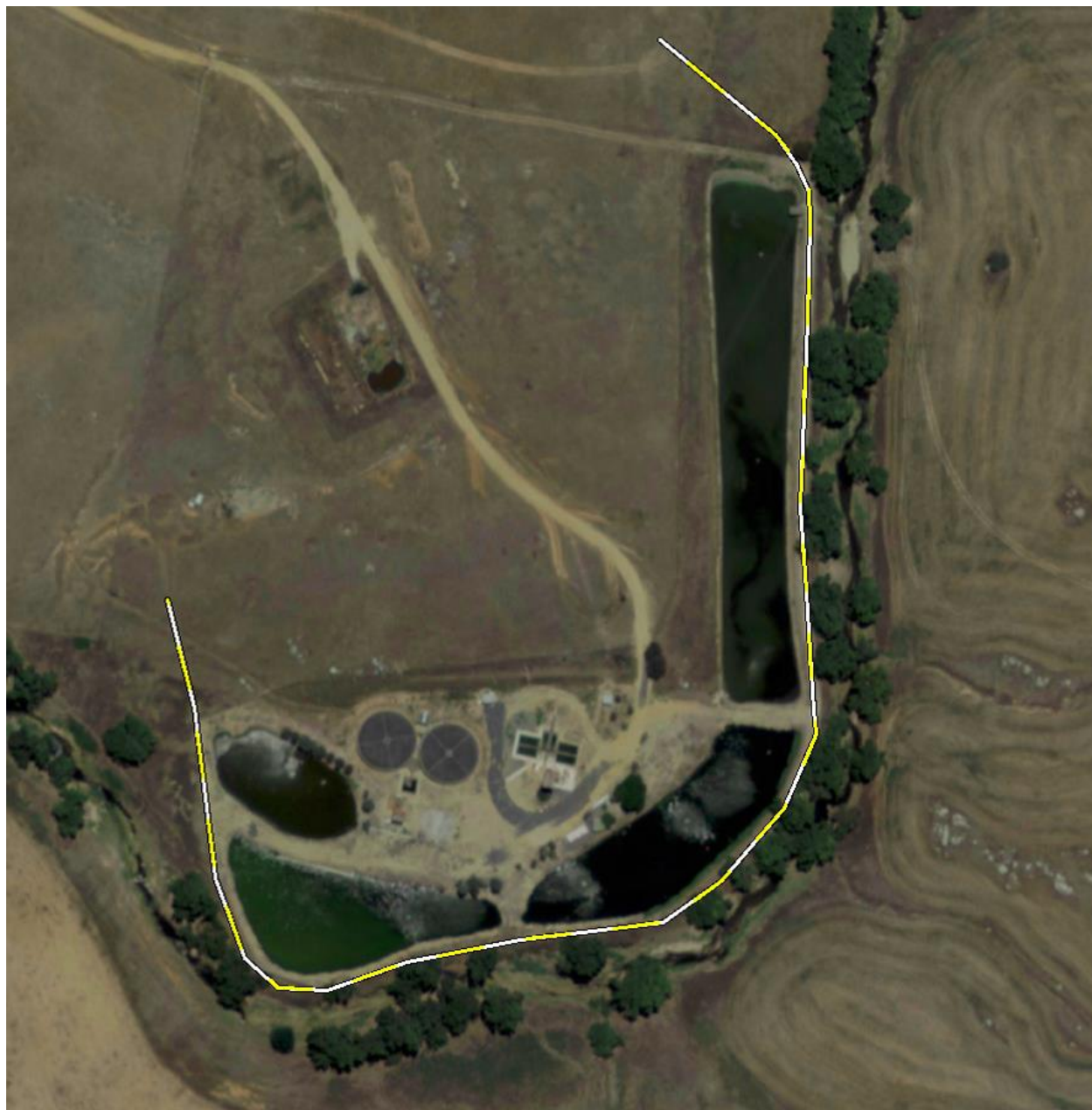
Diagram 17: Potential Sewage Treatment Plant Levee Alignment
